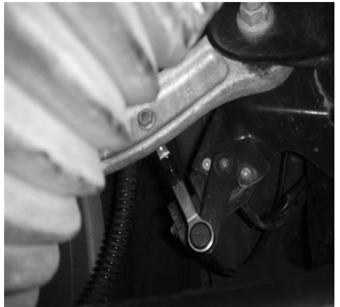
Adjustable Link installed
