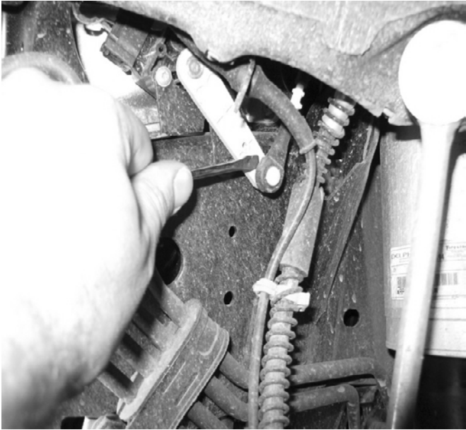
Front Stock Link removal
