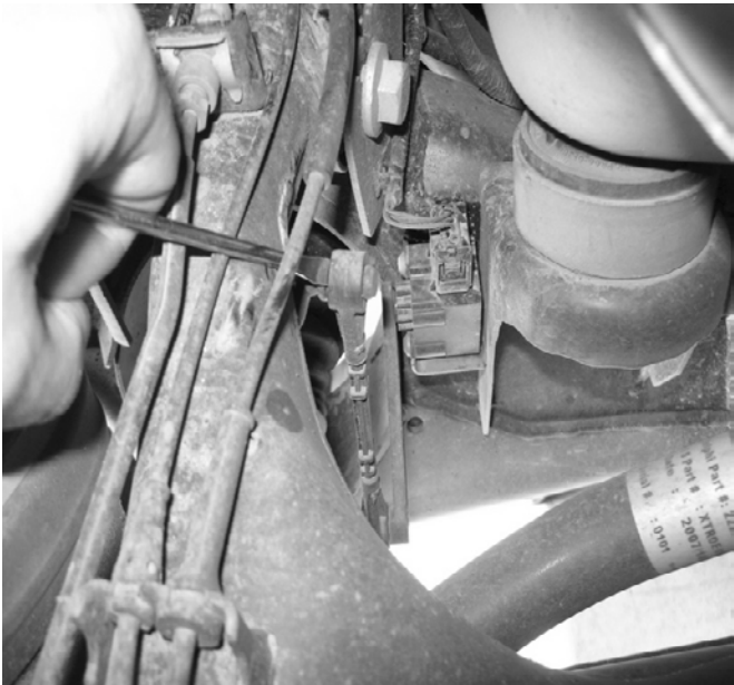
Rear Stock Link removal
