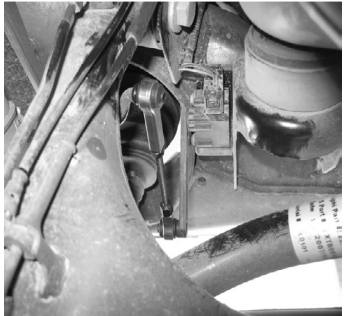
Adjustable Link installed
