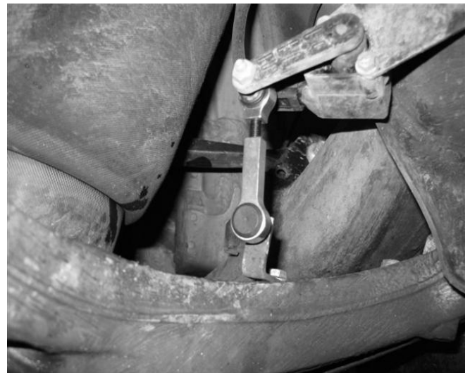
Rear Adjustable Link Installed
