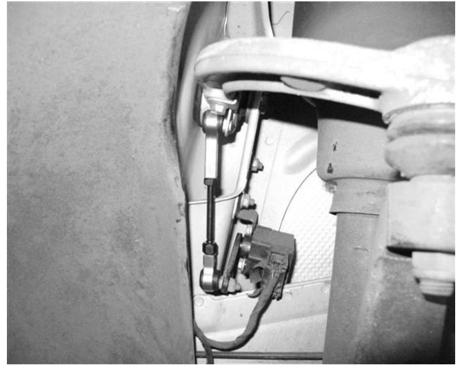
Front Adjustable Link installed
