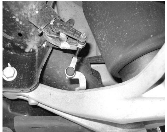
Rear Adjustable Link Installed
