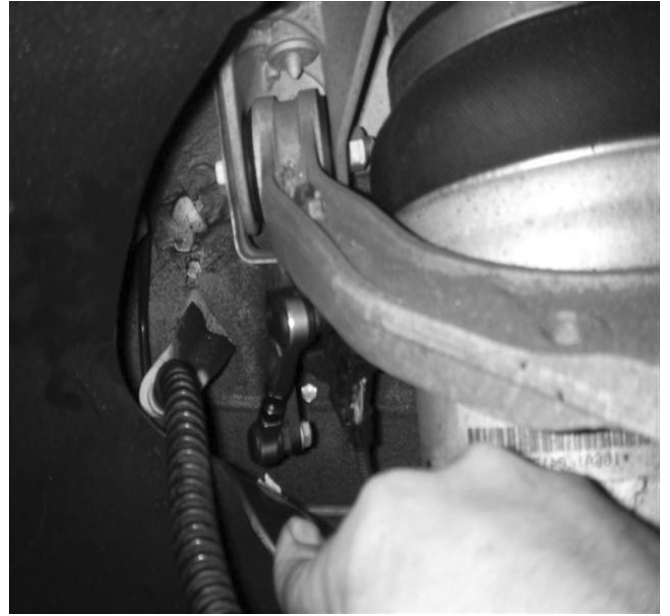
Adjustable Link installed
