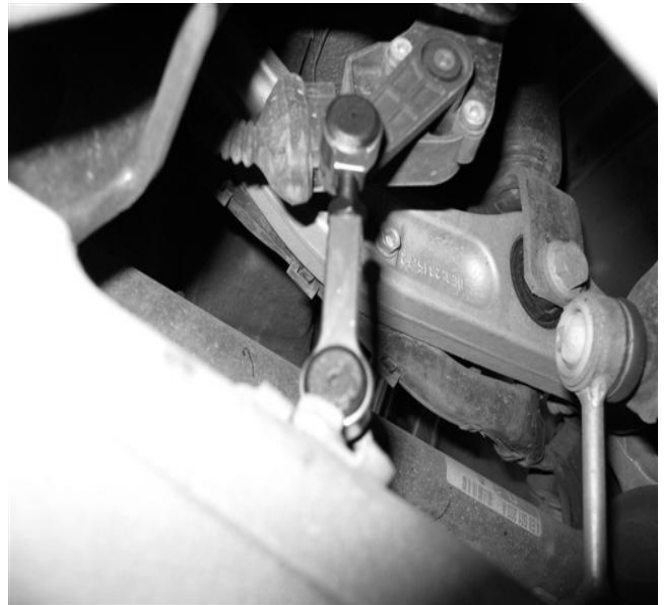
Adjustable Link installed
