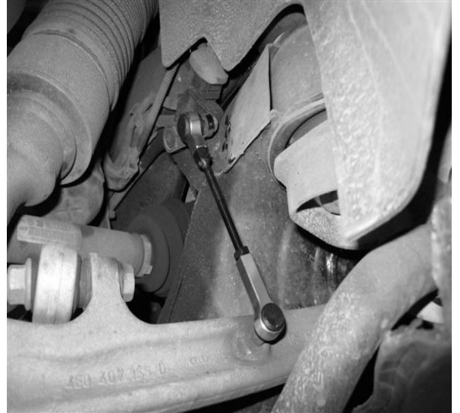
Adjustable Link installed
